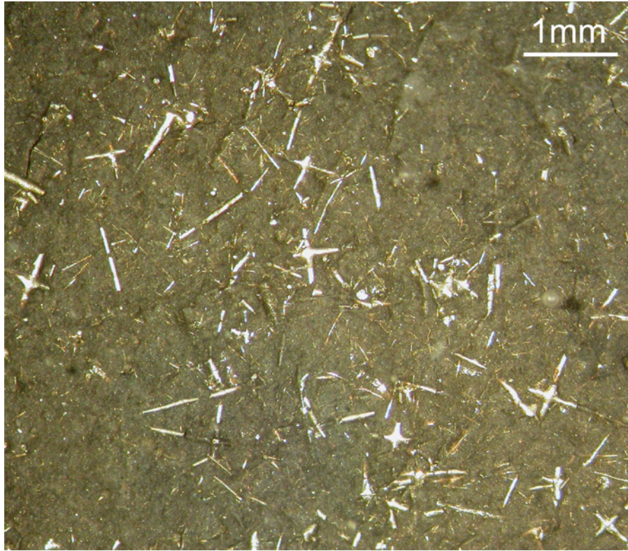
Figure N-20-15. Small pyritized sponge spicules, binocular microphoto of bedding plane, 1957.8 m MD; scale ruler on left in millimeters.
