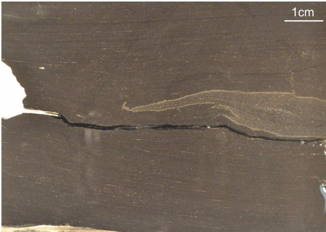
Figure N-20-12. Mudrock with carbonate stellate aggregates and a poorly formed pyritic-carbonate nodule, 1938.3 m MD
