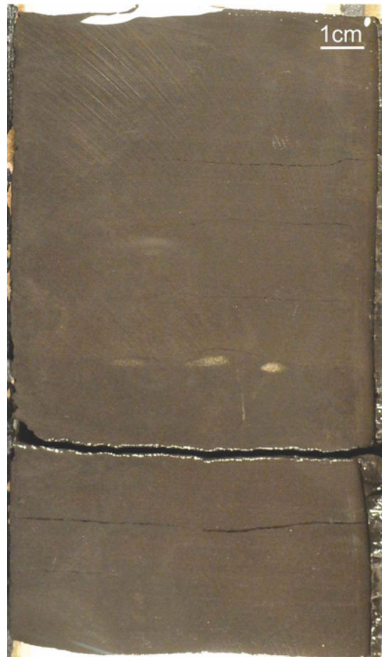
Figure N-20-11. Homogeneous subfissile mudrock with poorly formed small pyrite nodules in the middle, 1935.5 m MD
