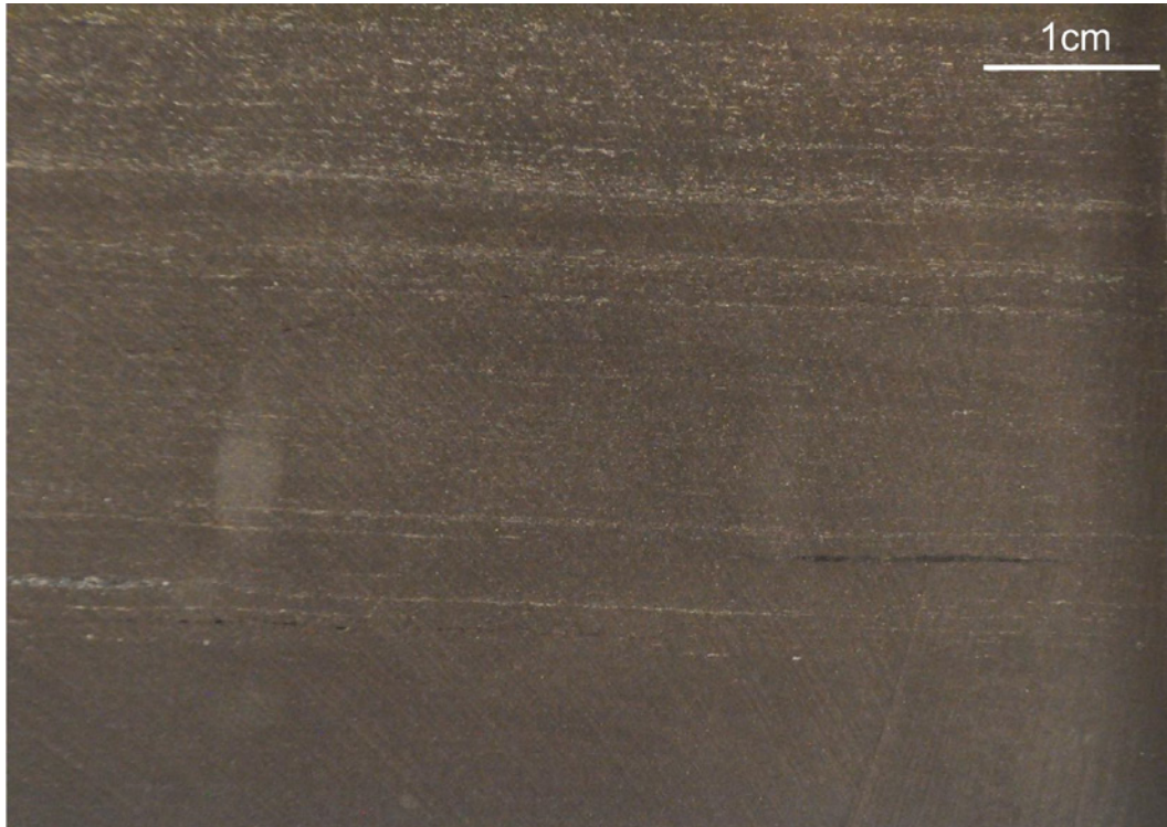
Figure N-20-10. Calcareous mudrock with calcisiltite laminae, 1935.1 m MD
