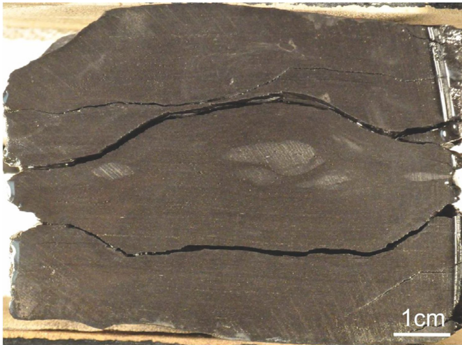
Figure N-20-14. Dark gray subfissile non-pyritic mudrock with small carbonate (siderite?) nodules, 1957.30 m MD
